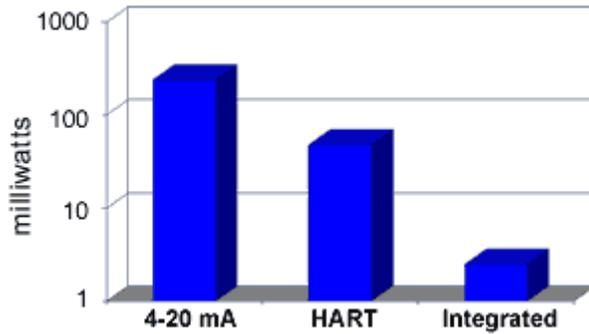
Integrated radio/sensor devices take advantage of low-power electronics to reduce energy consumption.
