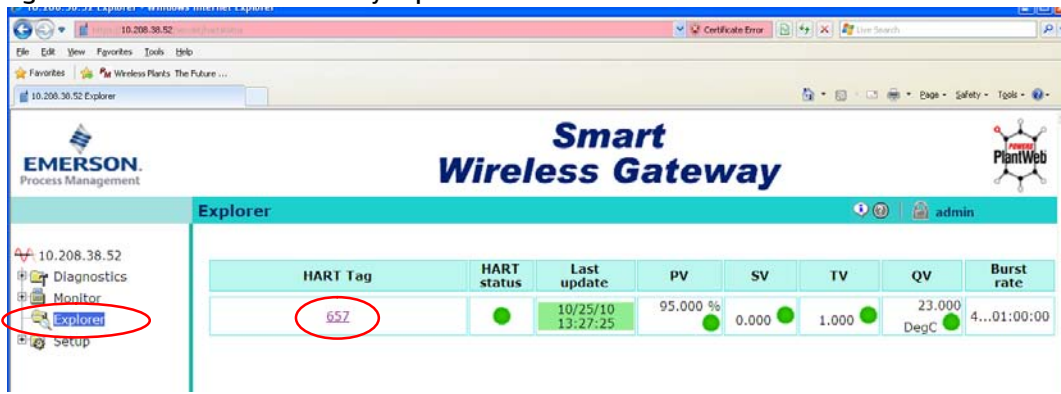
Figure 2. Smart Wireless Gateway Explorer
