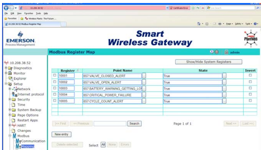
Figure 6. Mapping Modbus Data using Bit Data Values with Input Registers
