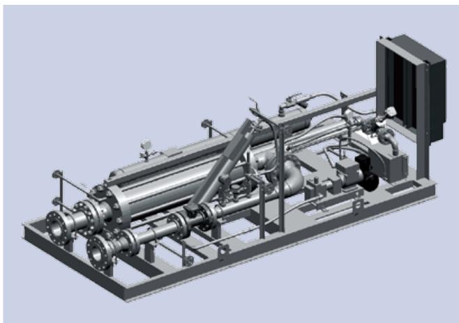
**FIG. 8** Small volume prover with turbine master meter.
