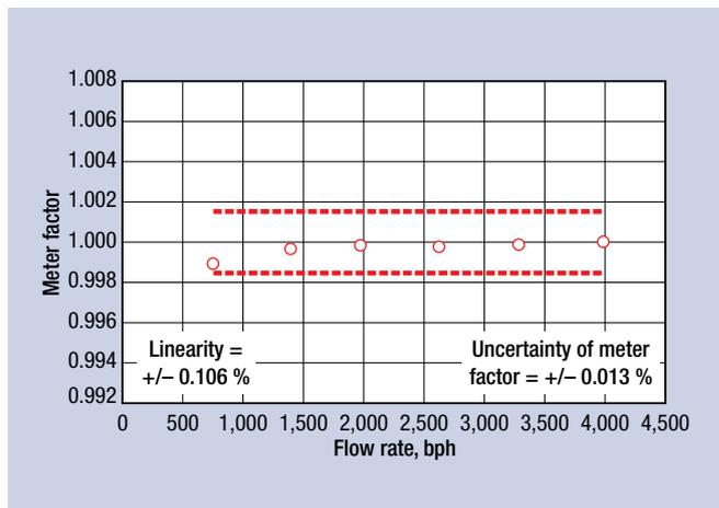
**FIG. 9** Liquid ultrasonic meter 6-in. calibration chart—using ball prover with ample volume.
