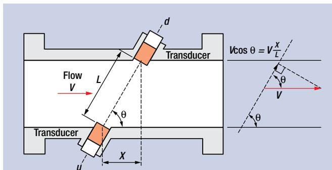
FIG. 2 Variables for calculating transit time.
