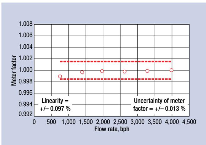
**FIG. 10** Liquid ultrasonic meter 6-in. calibration chart—using in-situ master-meter/small volume prover.
