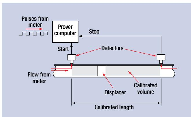
FIG. 3 Proving a meter by displacement.
