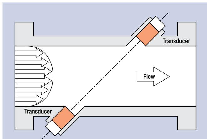
FIG. 1 Transit-time principle for ultrasonic flowmeters.
