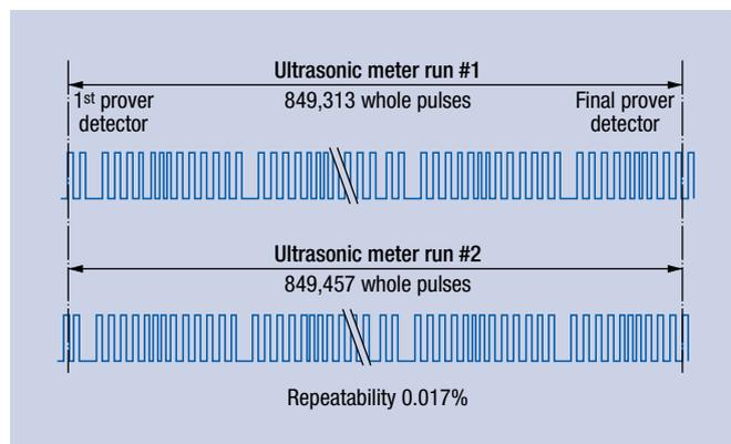
**FIG. 7** Typical proving results for ultrasonic meters using a larger proving volume.
