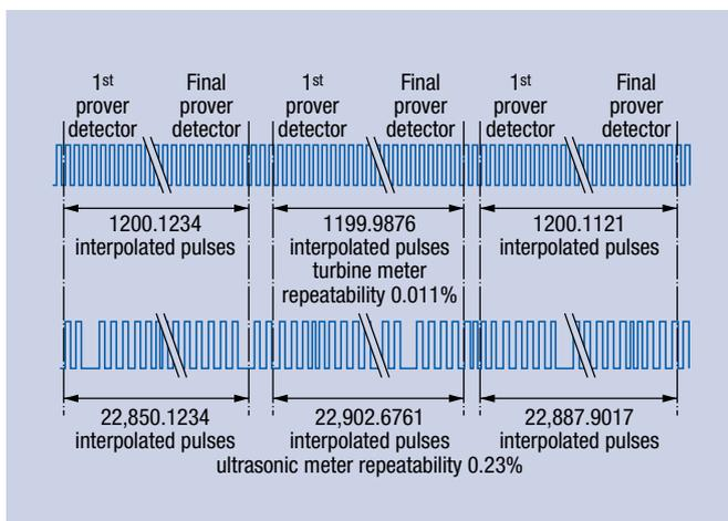
**FIG. 6** Typical proving results for turbine and ultrasonic meters using small proving volumes.
