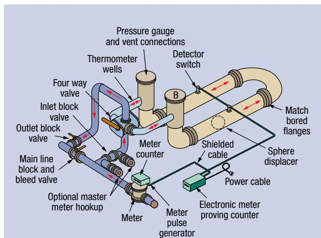
FIG. 4 A bidirectional ball prover.
