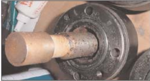
The dirtiest transducer was located closest to the bottom of the meter body and faced upstream.
