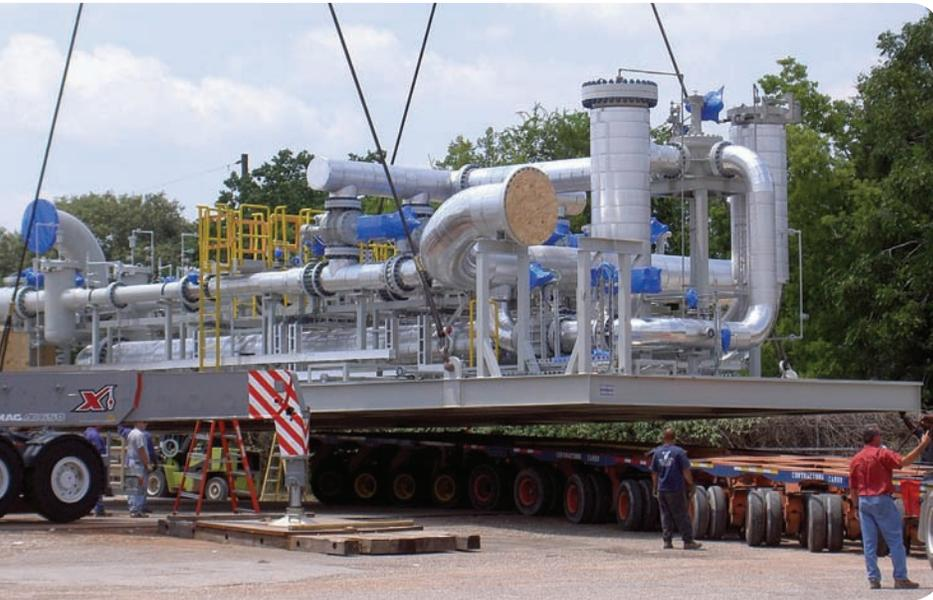
*This photo gives a better impression of how large and heavy (More than 40 tons.) a full-scale pipeline system can be. The fact that it may handle between \$5 and \$10 million worth of natural gas each day explains why accuracy and repeatability are so important. Error levels that would be tolerable in a process plant context can cost one side or the other tens of thousands of dollars in a matter of hours.*
