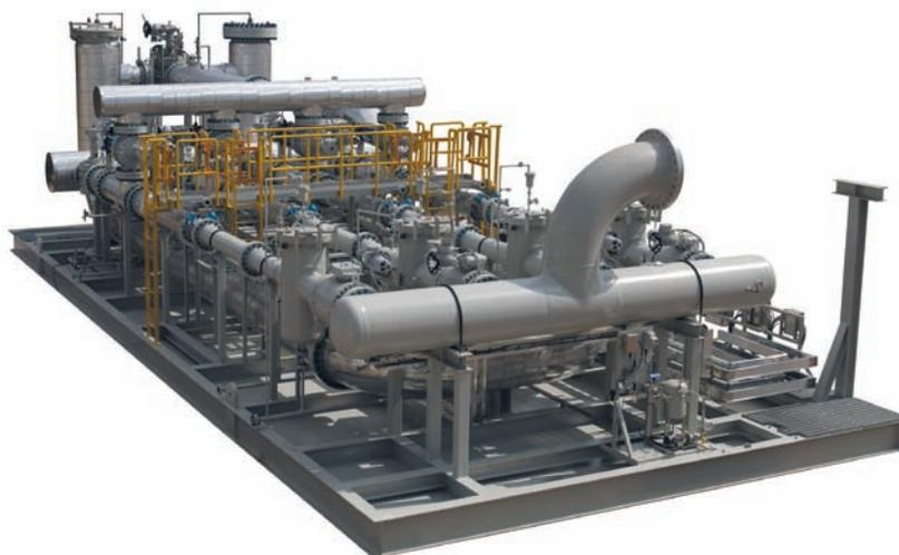
*Figure 4: Completed meter on a skid, ready for installation. The tubes are factory aligned meter-to-tube, conditioner plates and approach/discharge spools are concentrically aligned, and bolts are drawn up in sequence. All flowmeters, thermowells, analyzers and other equipment have been installed, wired and calibrated.*
