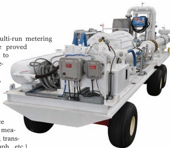
*Figure 3: A flow prover is installed in a custody transfer system to provide the most accurate measurement possible. It is used to calibrate the other flowmeters before, during and after a transfer.*
