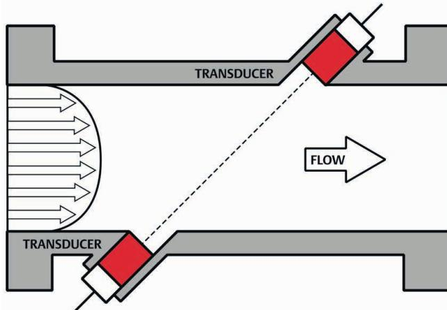
**Figure 3.** Ultrasonic instruments transmit and receive pulses diagonally across pipes to measure fluid flow.
