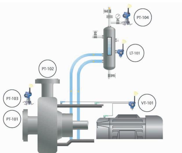
**Figure 2. Pump monitoring diagram.** A wide variety of parameters are typically measured on pumps used in pipelines, some of which are depicted in this diagram.
