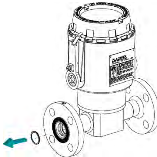
Figure 9-1: Retainer ring removal
