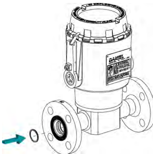
Figure 9-20: Sleeve and retainer ring installation
