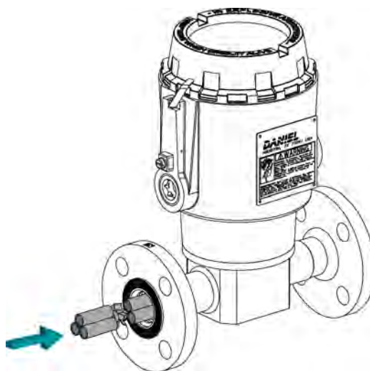
Figure 9-19: Internal assembly installation
