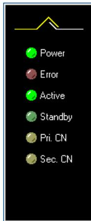
From DeltaV Diagnostics you can see the status of the active and standby OPC servers. Indication of the active and standby OPC server status is also available from a redundancy status faceplate display located in the system tray on the Application Station pair.
