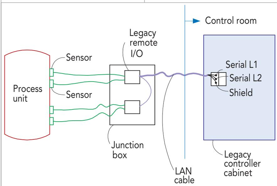
FIG. 1: Existing wiring shows analog connections from sensors to legacy I/O.
