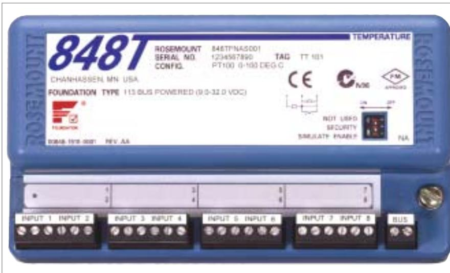
FIG. 2: The 848 temperature transmitter accepts up to eight analog inputs using the FOUNDATION fieldbus standard.
