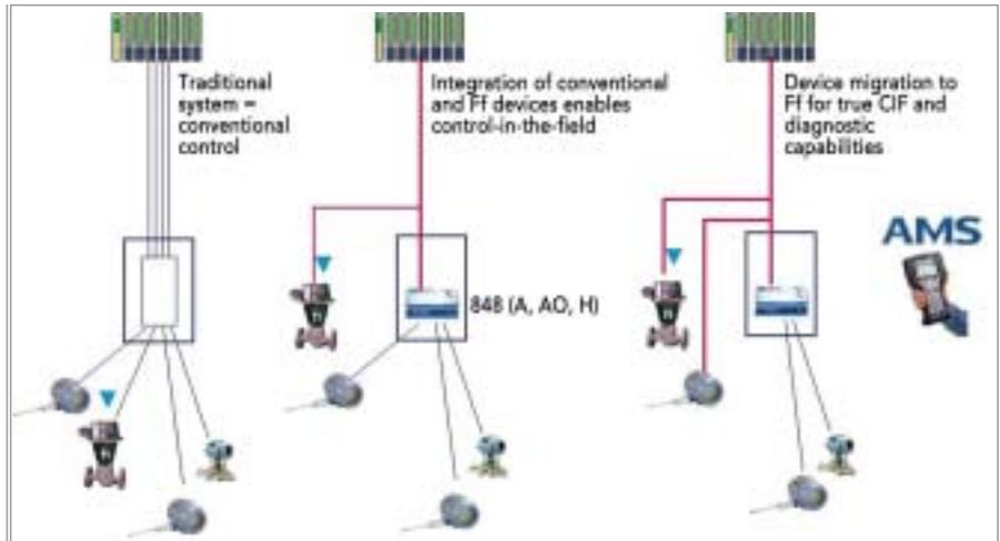
FIG. 3: A phased approach called for integrating analog instrumentation with the FOUNDATION fieldbus network.
