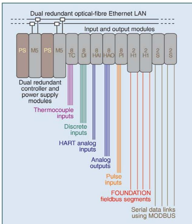
**Figure 5. Simplified diagram of the DeltaV controller for the naphtha stabiliser, illustrating modular construction and dual redundancy. If one controller, power supply or LAN fails, the other takes over without interrupting the service.**
