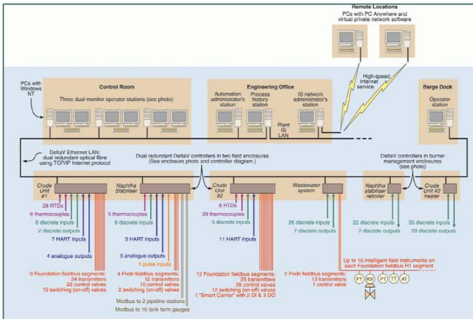
**Figure 3. Simplified diagram of the PlantWeb network as of July 2002.**
