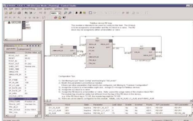
**Figure 9. In the friendly Windows environment, control connections and functions are configured by dragging and dropping with graphic tools as shown here.**
