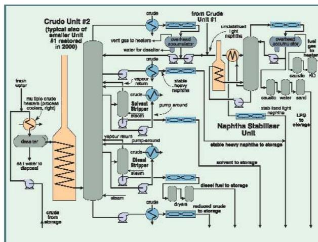
Figure 2. Simplified process flow diagram of Calcasieu refinery after Crude Unit 1 was restored in 2000, bringing the plants capacity up to 22 000 bpd.
