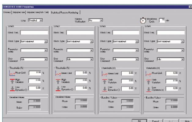
**Figure 10. A stage in advanced diagnostics of a transmitter with AMS.**
