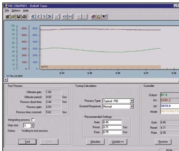
**Figure 12. Automatic tuning of control loops is built into DeltaV.**
