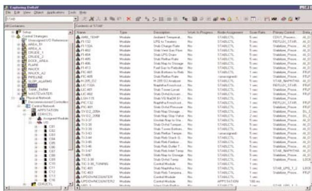
**Figure 8. When an intelligent instrument is first connected, it automatically appears as an icon on a Windows style DeltaV display such as this.**
