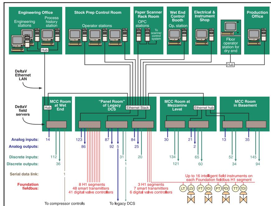
**FIGURE 2.** Simplified block diagram of the mill's digital automation system network. In two years, the digital plant architecture has replaced the legacy DCS everywhere but the powerhouse.
