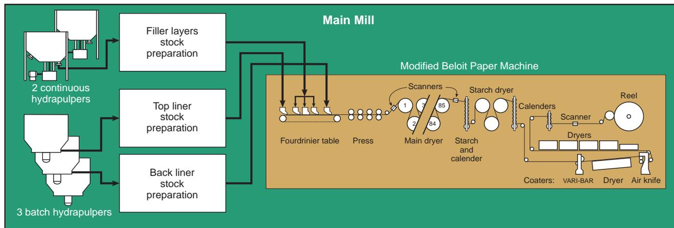
**FIGURE 1.** Simplified flow diagram for major components of the Sprague mill's stock preparation area and paper machine
