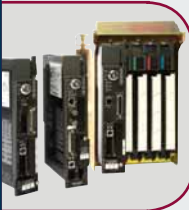
Rockwell PLC-5 controller
