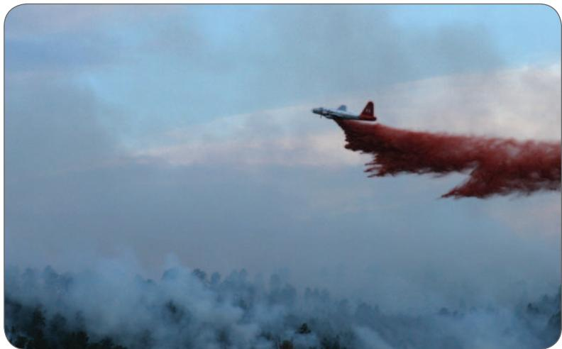
Figure 1. A PB4Y fire bomber drops Phos-Check on a brush fire. The bright red retardant fades in the sun and eventually decays into fertilizer.
