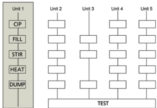
Figure 2. The vertical slice involves addressing one complete unit and all its associated control levels. Underneath are equipment modules with software blocks of code that operate equipment such as pumps and motors, agitators and such that are used in the processing of the pot. The control module is yet another lower layer of detail which handles all the various IO bits and pieces such as transmissions coming in, outputs to the control valves, and other control functions.
