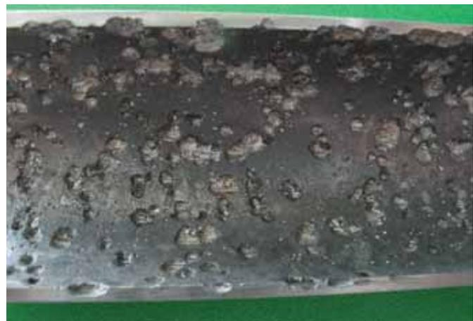
**Figure 1a.** This cross-section through a Ni-Cr-Mo alloy (UNS 06022) tube after exposure to a high concentration of hydrochloric acid resulted in large pits (2X).
