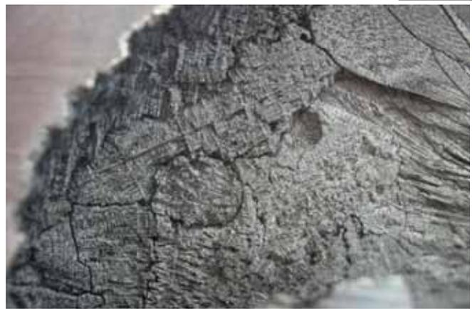
**Figure 2a.** This cross-section through a Ni-Cr-Mo casting (CW-2M) after exposure to nitric acid reveals the dendritic microstructure (1X).
