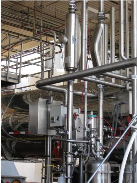
**Two-truck receiving bay using Micro Motion H300 flowmeters for direct mass measurement of delivered milk**
