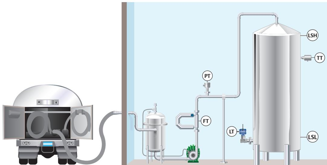
**Raw milk received from dairy farms must be monitored for quantity received, fat content and temperature during offloading to raw milk storage vessels**
