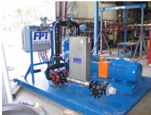
A full stream fluid density and flow rate skid system with a Micro Motion D300 meter installed
