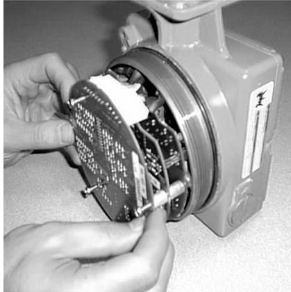
8. Unplug the wiring connectors as shown in Figure 3. Exercise care to avoid pulling the wires loose from the connectors.
