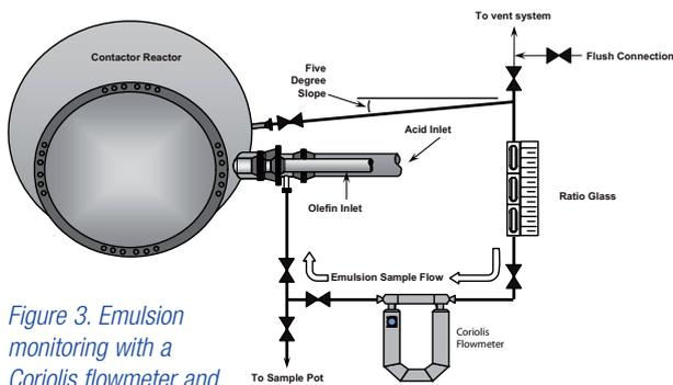
Figure 3. Emulsion monitoring with a Coriolis flowmeter and ratio glass.
