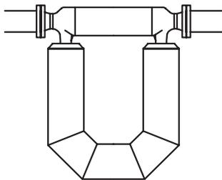
Figure 5. Best Coriolis flowmeter orientation.
