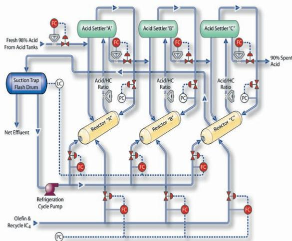
Figure 4. Coriolis flowmeters throughout the alkylation unit.
