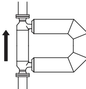
Tubes in "flag" orientation in vertical run (flow direction up)
