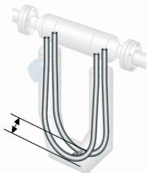
Figure 2. Coriolis flowmeter as a spring mass system.
