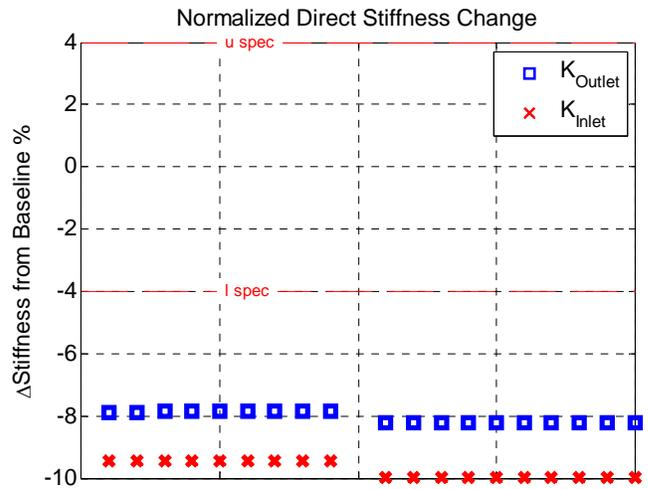
Figure 8. Direct Stiffness Verification - Eroded Meter
