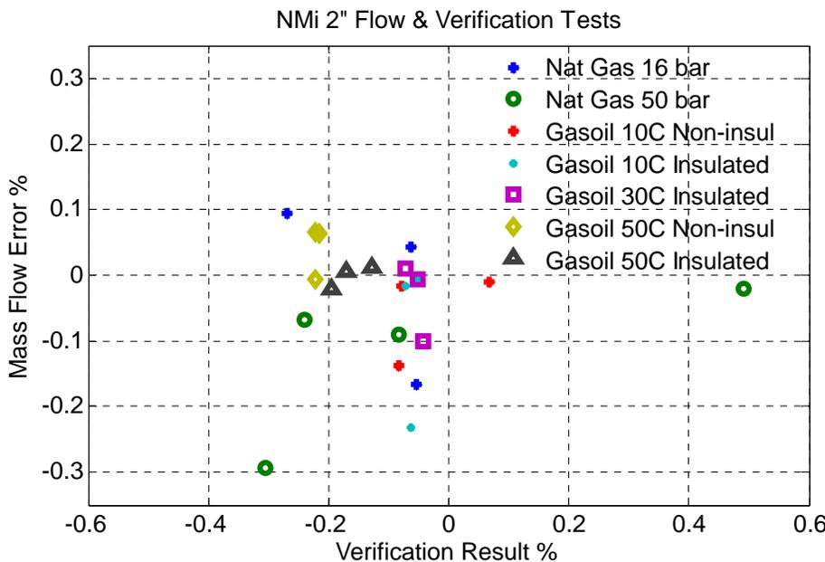
Figure 5. NMI Testing Mass Flow Accuracy vs Verification Results 2" meter
