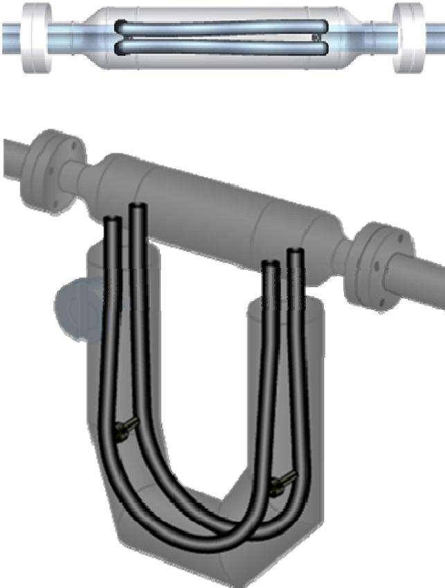
Figure 1. Typical Coriolis Meter
