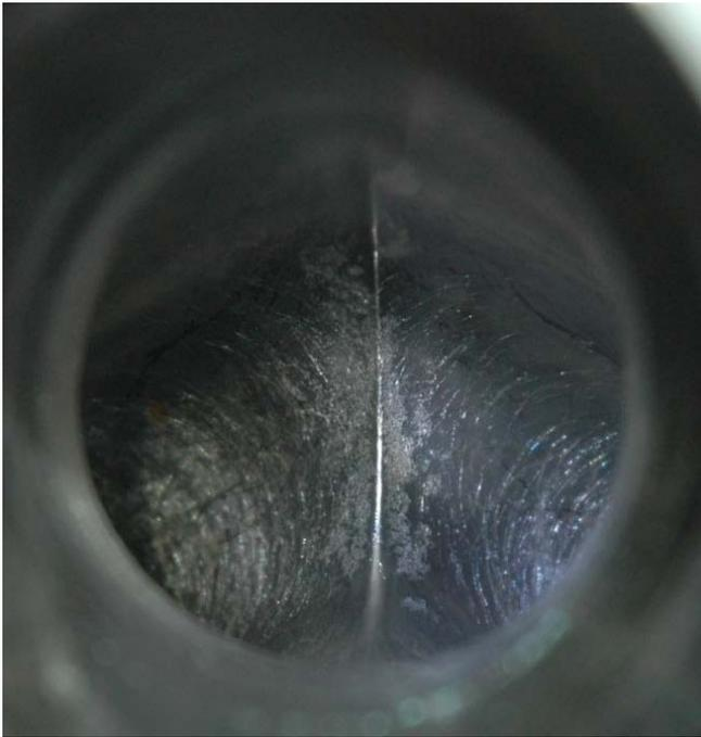
Figure 6. Eroded Inlet Manifold
