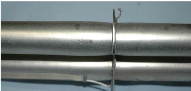
Figure 10. Over Pressurized Tube Failure
