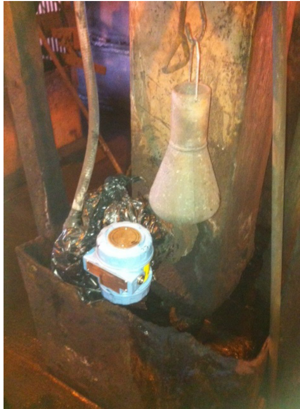
Micro Motion fork density meter controlling the magnetite slurry density
