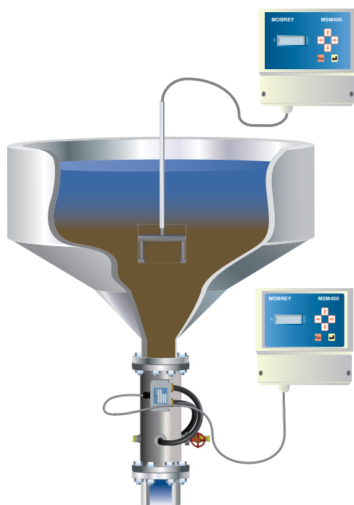
Robust stainless steel sensors may be tank mounted or housed in a pipe-section sensor on the clarifier
