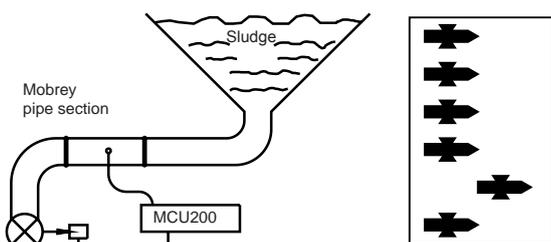
**Fig. 12 Sludge discharge control**
