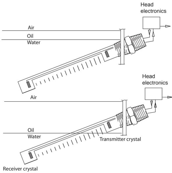
**Fig 14 Interface detector by reflection method**
