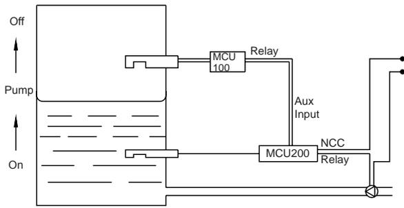
**Fig. 10 Tank filling pump control**
