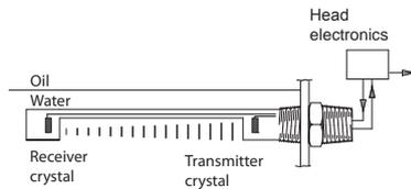
Fig. 13 Mobrey 402 sensor as oil/water interface
