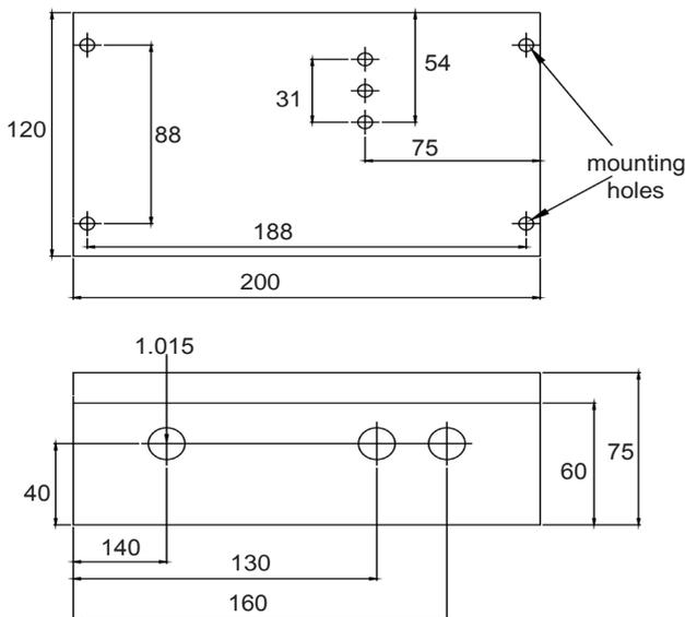
Fig. 3 MCU200 housing dimensions
