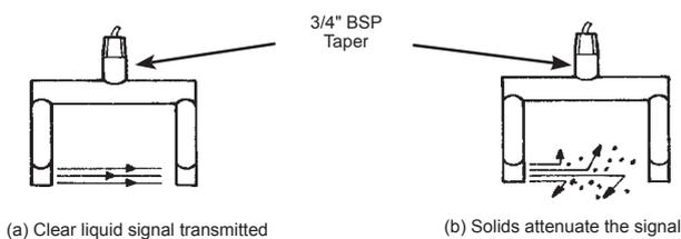
**Fig. 11 Type 433 sensor for suspended solids blanket alarm**
