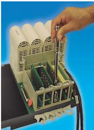
The replacement kit offers easy mounting or removal of the back-plane, personality cards, and electronics module.
