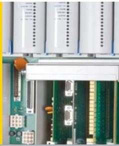
*The I/O migration program offers a one-for-one replacement of Q-Line I/O with Ovation I/O. Each Q-line card is replaced with a newly developed personality module and a standard electronics module. The card edge connector from the termination (“B”) cabinet plugs directly into the personality module, therefore preserving the existing field terminations.*
