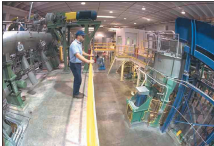
Figure 1. Pilot plant, Voith Paper Technology Center, Voith Paper Inc., Appleton, Wis. The control room is at the top of the stairs (center).
