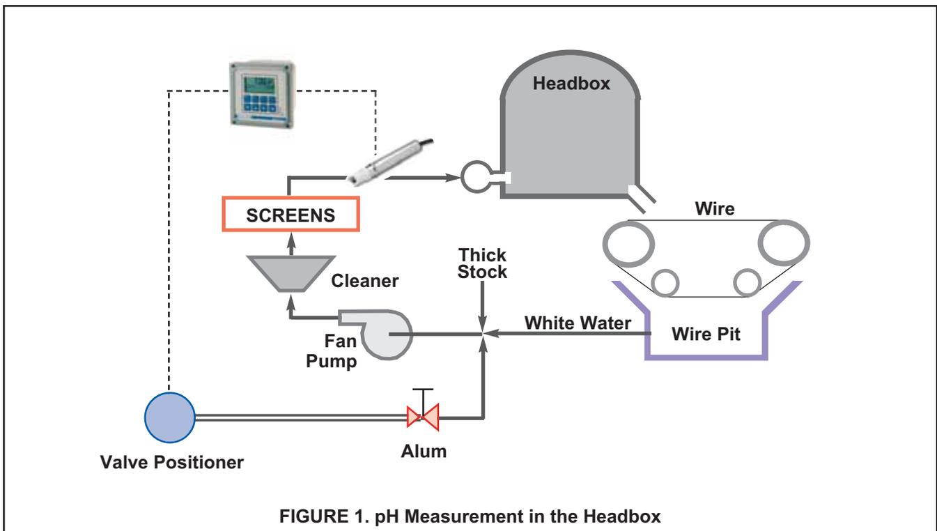
FIGURE 1. pH Measurement in the Headbox
