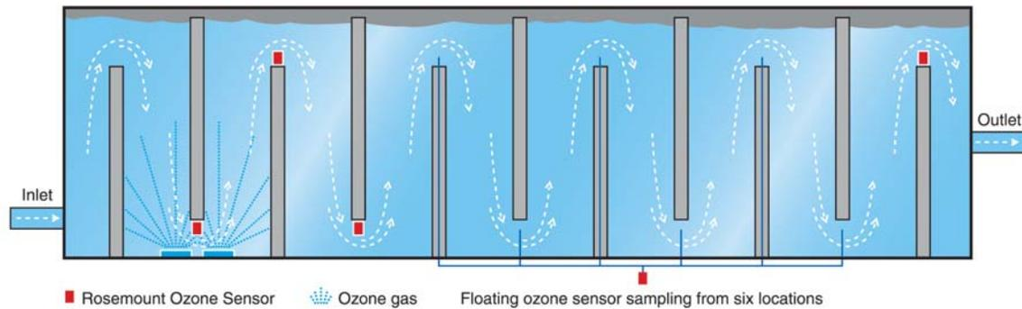
that survives less than 30 minutes. The rate of degradation depends on the water chemistry, pH and temperature. Because ozone is unstable, it is generated on site. Ozone is bubbled up through the water in contact chambers. By the time the water reaches the end of the contact chambers, primary disinfection is complete and the ozone has converted back to oxygen.
