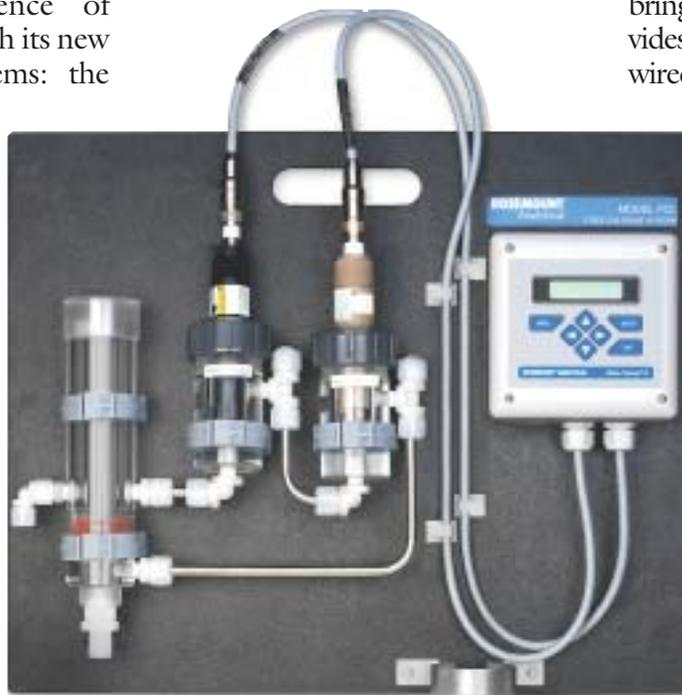
The Rosemount Model FCD system for free chlorine monitoring.
