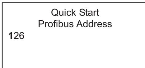
Enter a numeric Profibus network address from 000-125 for the Model 1056 Profibus device to be commissioned.
