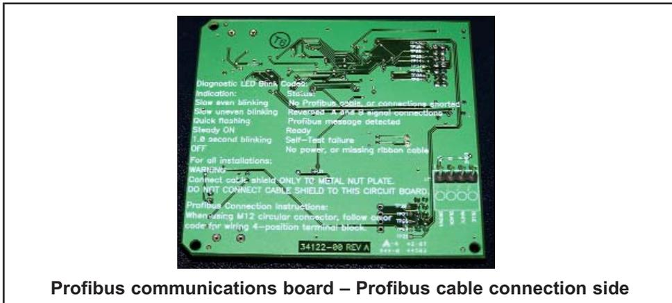
**Profibus communications board – Profibus cable connection side**
