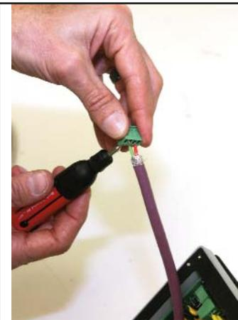
**Wiring Profibus cable to 4-lead terminal block**
