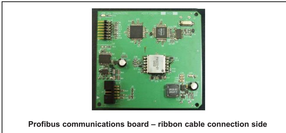
**Profibus communications board – ribbon cable connection side**
