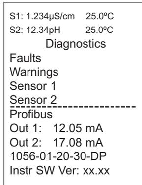
2. Scroll down and select Profibus. Press ENTER. Based on the condition of the Profibus installation and network connection, a number of diagnostics may appear.
