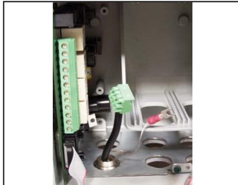
**M12 cable assembly wired to 4-lead Profibus terminal block.**
