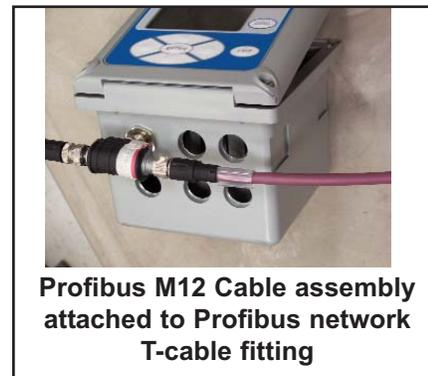
**Profibus M12 Cable assembly attached to Profibus network T-cable fitting**
