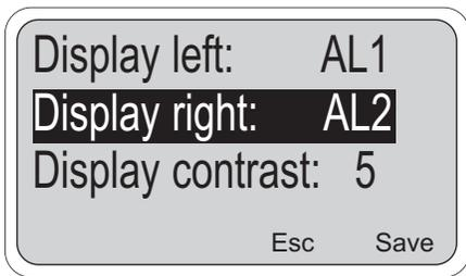
The "Display contrast" selection allows the display to be made lighter or darker. Entry 0 is the lightest and 9 is the darkest. The display changes as the number is changed.
