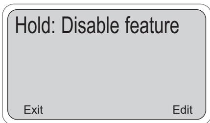
Press the Edit **[F4]** key to enable changes. Options include Disable, Enable, and 20 minute timeout. When 20 minute timeout is selected, the hold mode will automatically disengage after being on for 20 minutes. Selecting Enable or 20 minute timeout does not actually put the controller in hold, but rather allows putting the controller in hold when calibration is conducted.
