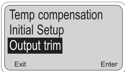
The instrument's current outputs may be calibrated (trimmed) if necessary. If either the power board or the CPU board is replaced, the outputs must be calibrated. To perform this procedure, a calibrated meter must be connected to the output being calibrated.
