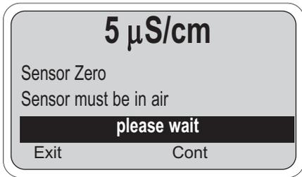
An unsuccessful zero will result if the conductivity reading is more than 1000 µS/cm or if the reading is too unstable. The "Zero offset error" message indicates the reading is too high for the zero routine. If repeated attempts do not result in an acceptable zero, there is a good chance that there is a wiring problem. Check Section 8.0, Troubleshooting, for help.
