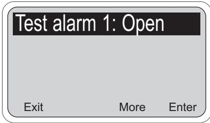
3b. The alarm relay is now being simulated. In the example to the left, alarm 1 has been set to Open. This means that the relay is not energized (i.e. off). The alarm will remain open until either Exit (F1) or Edit (F4) is pressed or the test is concluded by timeout. The default value for the timeout is 10 minutes, so after 10 minutes, the alarm would go back to normal operation and the display will return to the main menu. To configure the timeout option, see Section 5.5.
