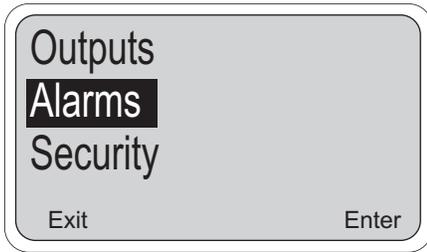
This section describes the options available for configuration of the alarms. Alarms 1, 2, and 3 can be activated on Conductivity (or resistivity, see Section 5.5), or temperature. One of these alarms can be setup as a feed limit timer and another alarm can be dedicated as an interval timer. Alarm 4 is reserved as a fault alarm.
