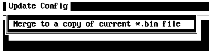
Figure 2. In the UPD_BIN program, choose "Merge to a copy of current *.bin file" from "Update Config" Submenu
