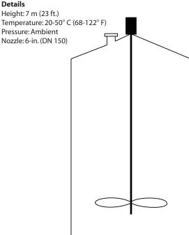
The radar gauge was mounted directly above the agitator blades. There were no problems with false echoes from the blades.
