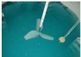
Inside the tank with the agitator and baffles to generate turbulence and the mechanical float gauge on the right.
