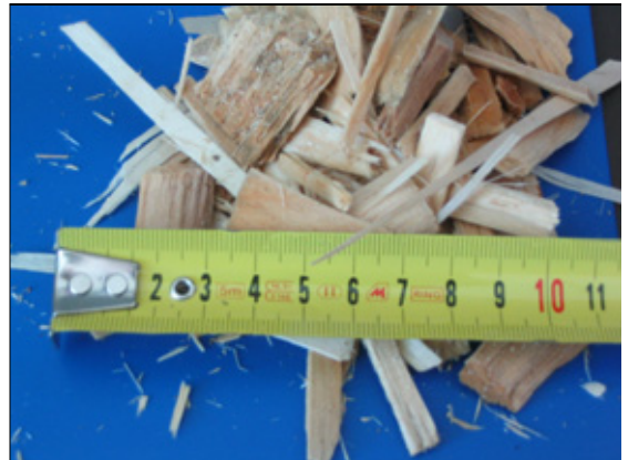
A sample of the wood chips. Note: The ruler is in centimeters.
