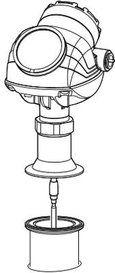
3. Tighten the clamp to the recommended torque (see the manufacturer's instruction manual).
