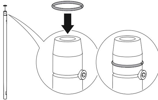
3. Optional: If ordered, mount the centering disc on the bottom segment of the probe.
