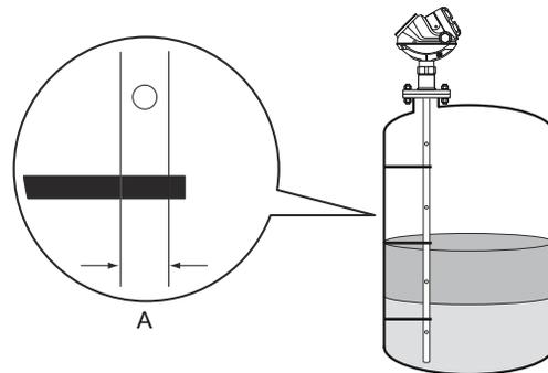
A. Coaxial:  $\varnothing$  1.1 in. (28 mm), Large coaxial:  $\varnothing$  1.7 in. (42 mm)
