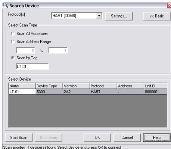
4. Ensure the Rosemount 5300 is alone on bus. Disconnect or turn off power from any other devices.
