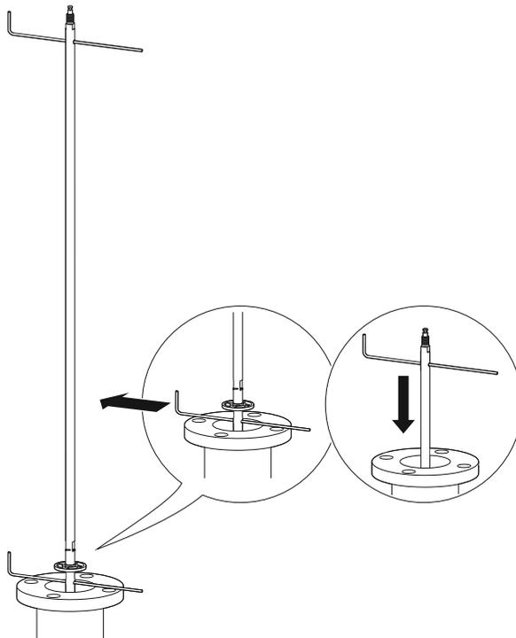
10. Repeat [Step 5-Step 9](#) until all segments are mounted. Be sure to finish with the top segment of the probe.
