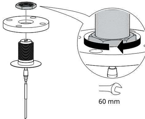
2. Place a suitable gasket on top of the tank flange.
