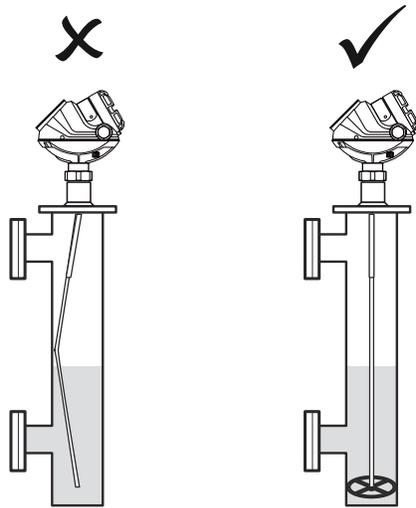
For the segmented rigid single lead probe, up to five PTFE centering discs can be mounted along the probe, but keep a minimum distance of two segments between the discs. Additionally, a disc in SST or PTFE (part number 03300-1655-xxxx) can be attached to the end of the probe.
