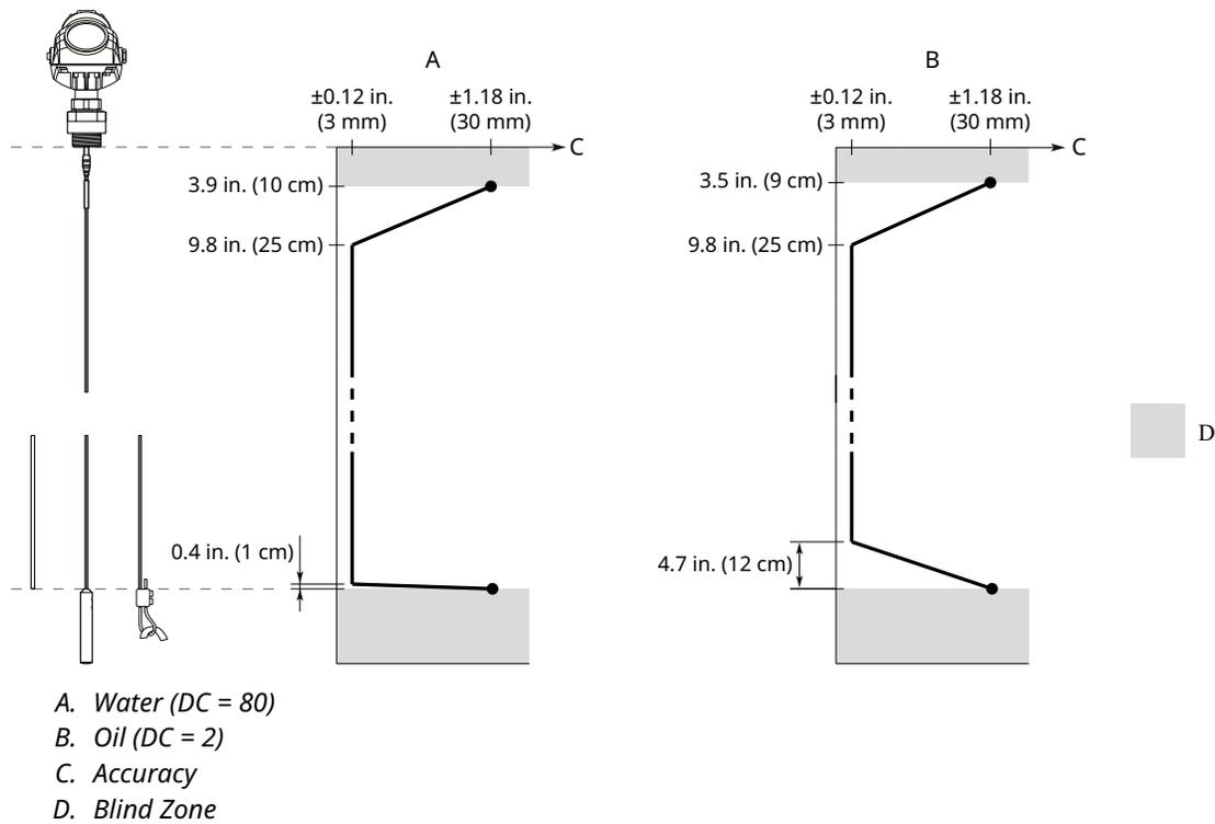
Figure A-5: Accuracy Over Measuring Range for Twin Lead Probes
