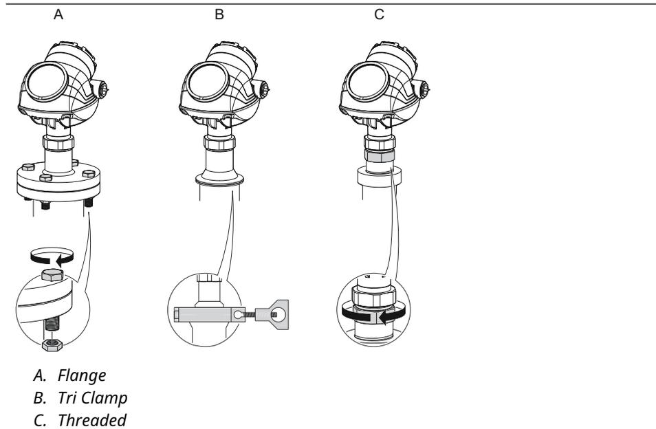
16. Rotate the housing to the desired direction.
