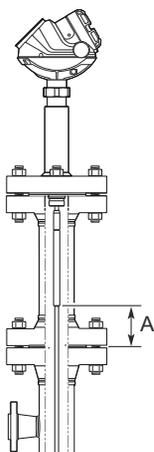
A. For the 4U probe, the spool piece needs to be at least 2 in. (50 mm) longer or shorter than the reference reflector.
