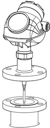
3. Tighten bolts and nuts with sufficient torque for the flange and gasket choice.
