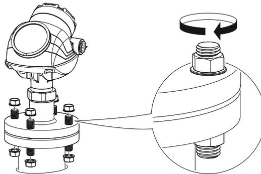
4. Loosen the nut that connects the transmitter head to the probe slightly.
