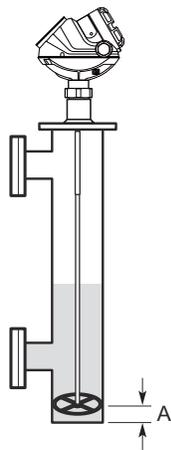
A. A clearance distance of 1 in. (25 mm) between the probe end and the chamber bottom is recommended.
