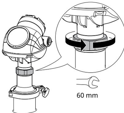
5. Rotate the transmitter housing so the cable entries/display face the desired direction.
