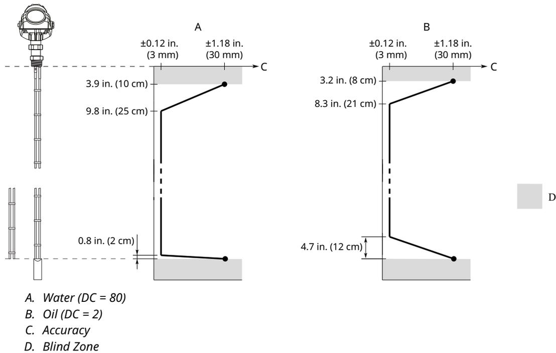
Figure A-6: Accuracy Over Measuring Range for Coaxial Probe
