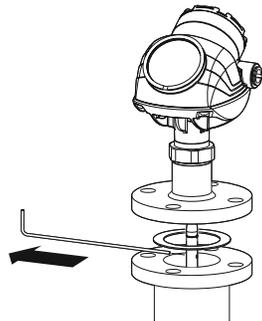
15. Mount the device on the tank.
