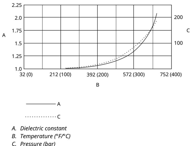
The standard version of a Rosemount 5300 Level Transmitter can be configured for static compensation of vapor by manually entering the dielectric constant of vapor. For applications with a varying pressure and/or temperature, certain models of the Rosemount 5300 have a built-in function (Dynamic Vapor Compensation) that automatically compensates for varying vapor dielectric constants.
