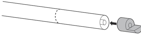
3. Cut the tube to the desired length.
