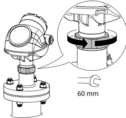
5. Rotate the transmitter housing so the cable entries/display face the desired direction.
