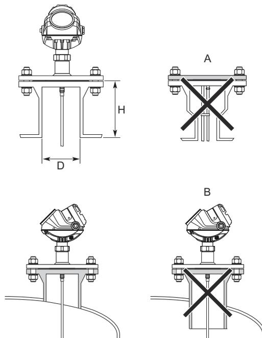
A. Avoid nozzles with reducer (unless using coaxial probe).
