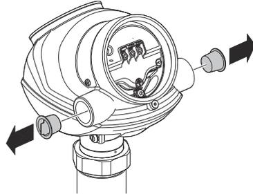
4. Pull the cable through the cable gland/conduit.
