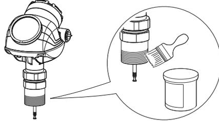
12. Attach the probe to the device.
