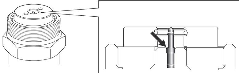
5. If the transmitter head is not mounted directly, attach the protection plug to the process seal to protect the exposed parts from dust and water. If a protection plug is not available, then cover the process seal with a plastic bag.
