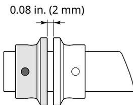
4. Insert the split pins through the bushings and the probe.
