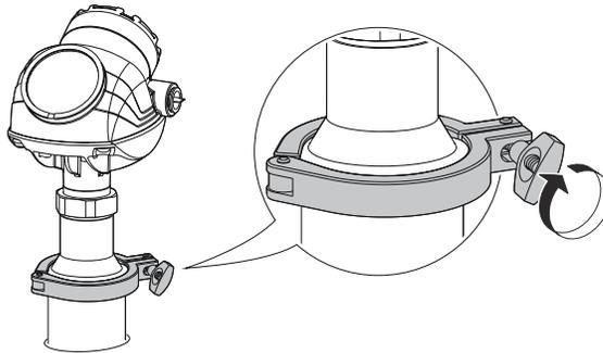
4. Loosen the nut that connects the transmitter head to the probe slightly.
