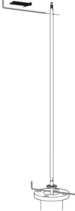
9. Remove the first support tool and lower the probe into the tank.
