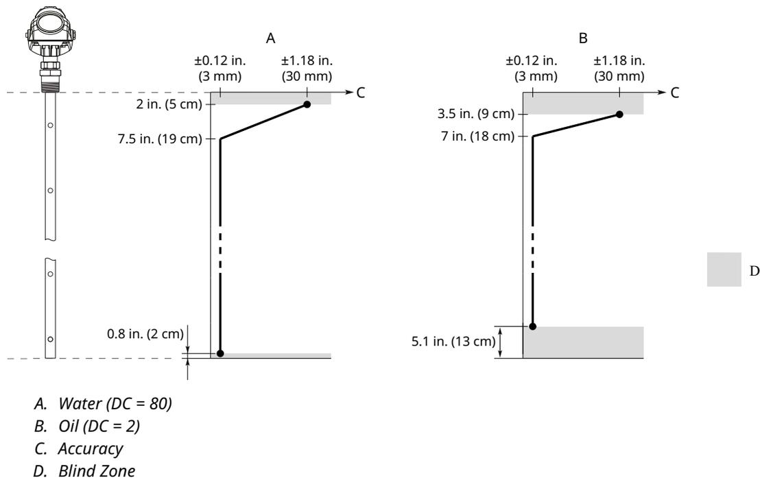
Figure A-7: Accuracy Over Measuring Range for Large Coaxial Probe
