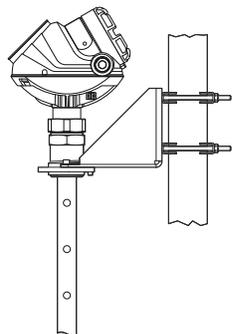
For optimal single lead probe performance in non-metallic tanks, the probe must be mounted with a metal flange, or screwed in to a metal sheet ( $d > 14$  in./350 mm) if a threaded version is used.
