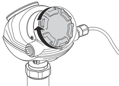
10. Turn the jam screw counterclockwise until it contacts the cover.
