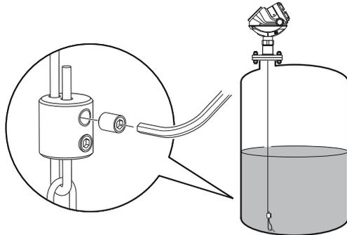
A ring (customer supplied) can be attached to the weight in a threaded (M8x14) hole at the end of the weight. Attach the ring to a suitable anchoring point.
