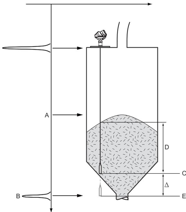
The product Level is given by the relation between Probe End displacement  $\Delta$ , the Dielectric Constant of the product, and distance D.
