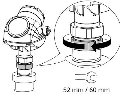
6. Rotate the transmitter housing so the cable entries/display face the desired direction.
