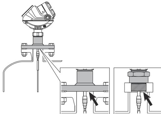
For standard tank connection, final rating may be lower depending on flange, material of construction, and O-ring selection. [Table A-10](#) gives the temperature ranges for standard tank seals with different O-ring materials.
