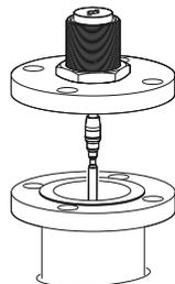
4. Tighten bolts and nuts with sufficient torque for the flange and gasket choice.
