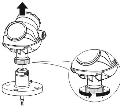
2. If installing a new unit, mount the probe on tank.
