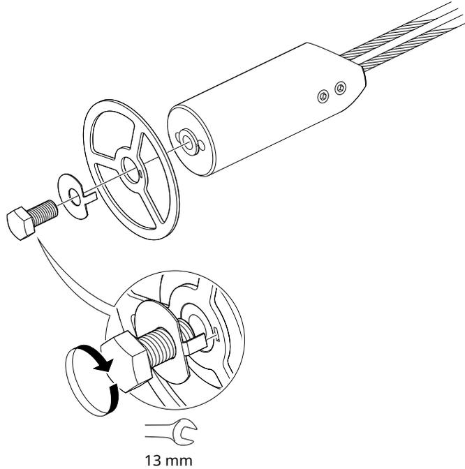
2. Secure the bolt by folding the tab washer.
