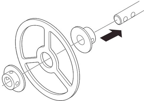
3. Adjust distance by shifting hole for split pin in lower bushing.
