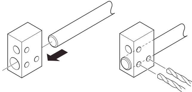
2. Mount the bushings and centering disc at the probe end.
