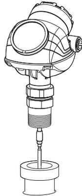
4. Loosen the nut that connects the transmitter head to the probe slightly.
