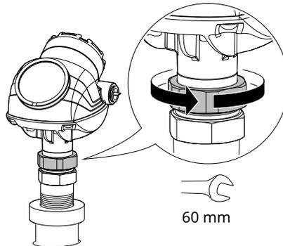
5. Screw the adapter into the process connection.
