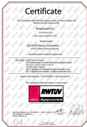
Figure 5: Certificate example for a sensor certified by TUV, the listed sensor complies to the requirements listed in IEC 61508 sections 2 & 3
