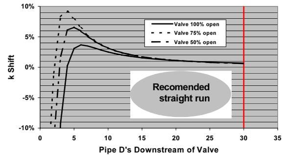
Figure 6: Butterfly Valve Errors Parallel to Valve Axis
