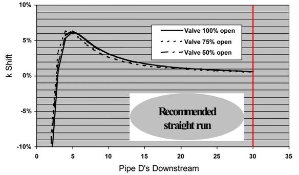
Figure 5: Butterfly Valve Errors 90° Off Valve Axis
