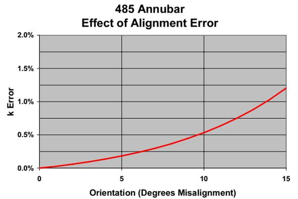
Figure 2: Effect of Alignment Error
