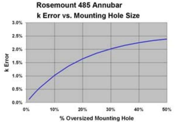
Figure 1: K Error vs. Mounting Hole Size
