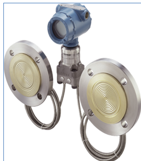
Figure 3 – A Balanced System has identical diaphragm seals and equal lengths of capillary on both the high and low sides of the DP transmitter.
