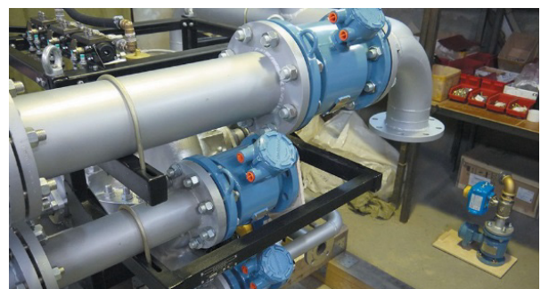
Rosemount Magnetic Flowmeters measure water and foam agent flow rate in fire engines with a capacity of up to 200 liters per second.
