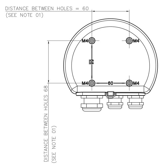
01 DRILL PATTERN FOR MOUNTING OF WEATHER PROTECTION.
