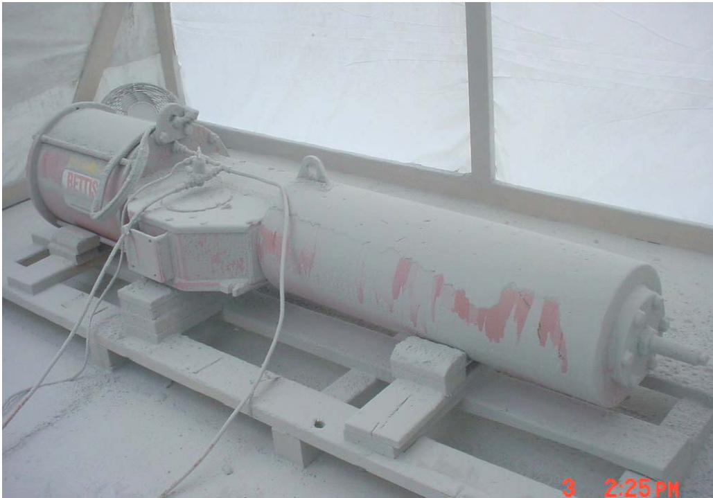
Photograph 5. Specimen View at the End of Dust Test
