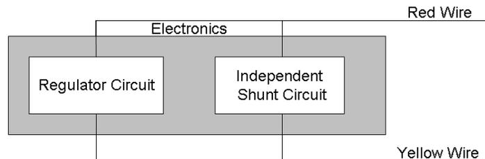
**Figure 3. How Loop Current Flows Through a THUM Adapter**
