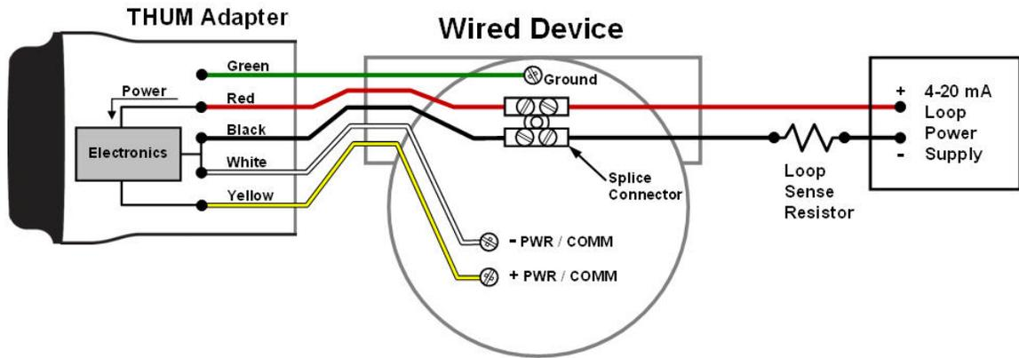
Figure 4. Wiring Diagram for THUM Adapter on a Two Wire Device
