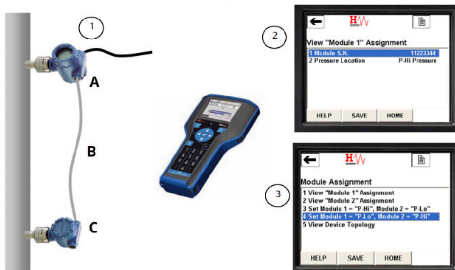
Figure 2-6: Example of How to Change the P HI and P LO Module Assignments
