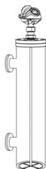
A centering disc helps to keep the probe away from the chamber walls. It is recommended for single rigid probes. Its applicability with long flexible probes is more limited.
