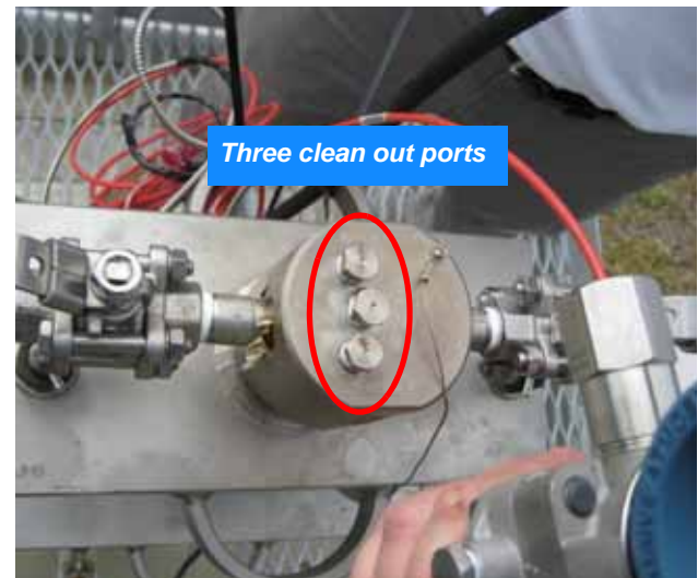
Figure 3. Clean out ports are in the head with large passageways to ensure easy maintenance and cleaning.
