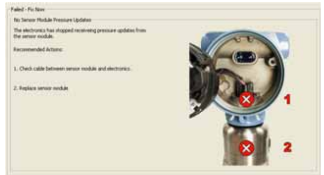
FIGURE 2. Graphically based troubleshooting and repair reduce time needed to resolve issues and reduce errors and rework.
