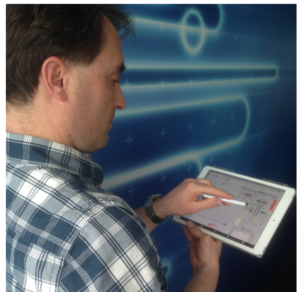
Ruggedized Apple iPad4 tablets with the DeltaV Remote Operator Station application.
