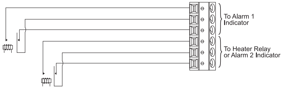
Figure 2-15. Alarm Indicator Relay Terminals
