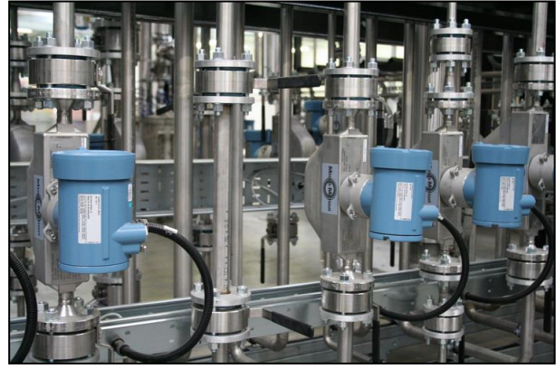
2/ IN ADDITION TO THE VALUE OF THE MASS FLOW, THE MICRO MOTION FLOW METERS CAN MEASURE VOLUME FLOW, DENSITY, CONCENTRATION AND TEMPERATURE, ALL WITH A UNIQUE INSTRUMENT
