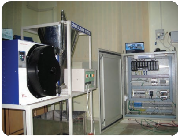
Figure 1. Conical Tank in MIT Anna University Lab with an industrial DCS.
