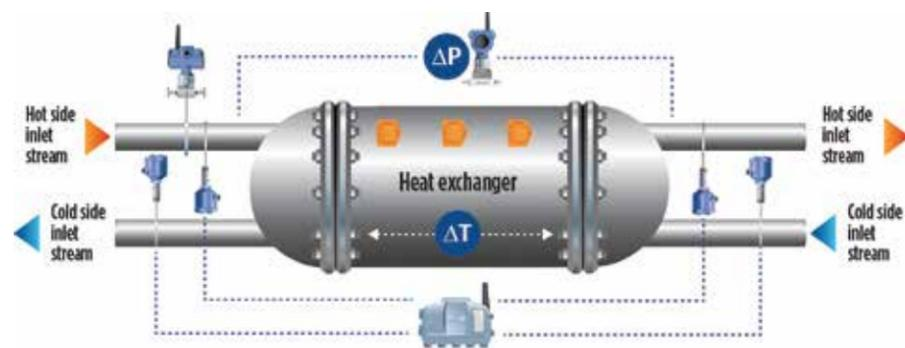
FIG. 2. Wireless transmitters on a heat exchanger.
